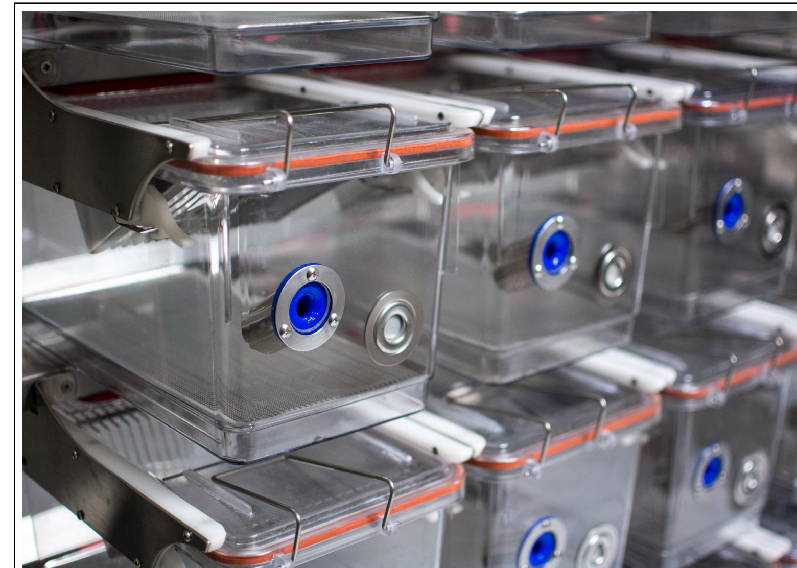
Figure 2: Front of the cage with out of the cage water bottle supports (blue) and the sampling port (grey).
