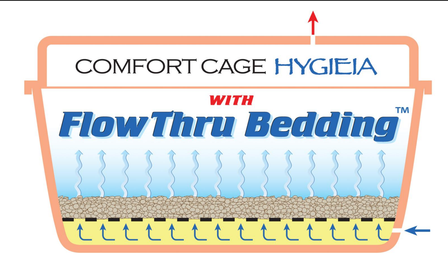
Figure 1: Schematic of the Lenderking IVC design, brand named Hygieia
